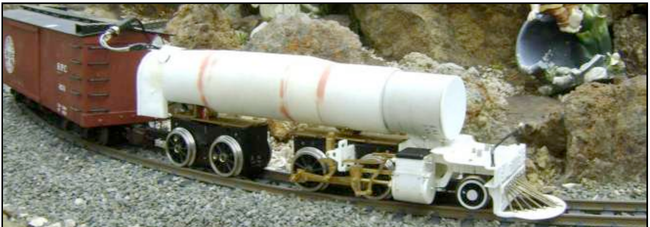
The first test run, plugged into a battery wagon delivering 7.2v direct to the two motor blocks.
