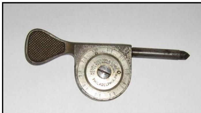
with the counter. Those who work with saws know that the rpm or more importantly the speed of the teeth cutting the wood is absolutely critical. This would be the reason that Disston's made their own rpm counter.
