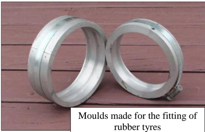
Moulds made for the fitting of rubber tyres
