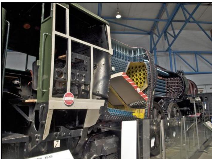
one of them has the boiler, cylinders and valve gear sectioned.
