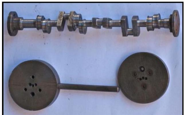
Shaft #4 together with the two end caps showing the centres of rotation.
