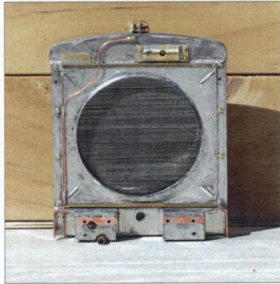
Front and rear views of the radiator and below the radiator fitted on the tractor. The radiator was constructed from tin-plate with some brass components. 10 - 10BA bolts hold the radiator onto the tractor.
