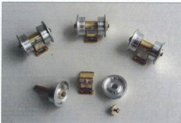
Construction of the top track rollers
