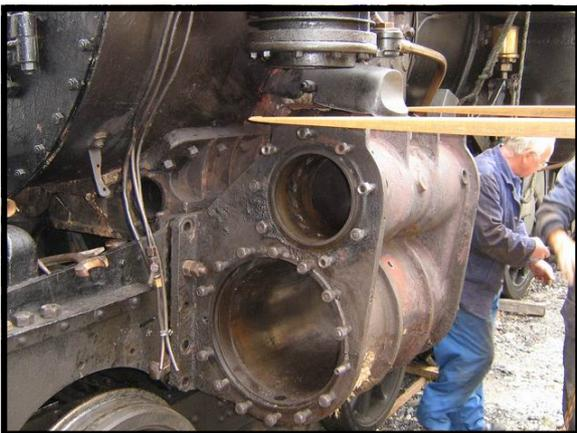
frame are fitted to reamed holes and are driven into place with a SledgeHammer. This meant that there was considerable difficulty in removing the bolts, as it was not possible to swing a sledgehammer between the frames because of the proximity of the saddle and other castings.
