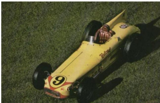
corners on to the long straights, the Ferrari got 'blown away' by the 4 cylinder Offenhauser. The picture is of the Belond Special built by George Salih for the 1957 'Indy 500' which it won. The same car won the 1958 race as well. It was powered by an Offenhauser laid over at an angle of 18 degrees. This was to lower the centre of gravity and give the car a smaller frontal area.
