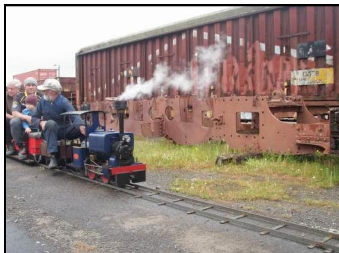
Of interest also alongside our track were the frame's of a "V" class 2-6-2 tender locomotive from the mid 1880's. These were built by Nasmyth Wilson in the UK and arrived in NZ grossly overweight. They spent time in Addington workshop's on a weight reduction diet before being allowed out onto the rails. I'm of the opinion that these locomotives formed the basis of our own NZR "W" class 2-6-2 Tank Loco's to which I am familiar. The "W" frames and gear being a direct copy of the "V's".
