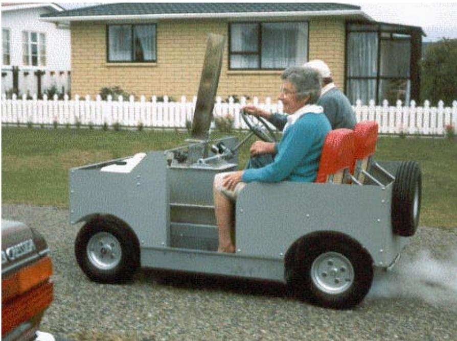
In 1992 I completed a task that had been a dream for many years. This was the building of a steam car. It had a duplex engine with cylinders of 1.625" bore and 2" stroke. The piston valves were actuated by Hackworth/ Marshall valve gear. The mono tube steam generator deliver steam at up to a maximum 600psi.
