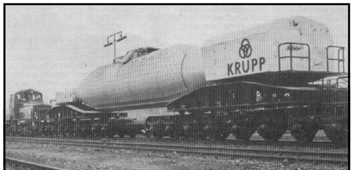
With a starting temperature of 1,400 C, the load only loses 5 C during the transit period. The container is emptied by rotating on its axis by electric motors in the end trucks. It takes just 4 minutes to empty the molten metal. In 1969 molten metal wagons were introduced in Britain. Three specially designed torpedo shaped wagons began a 63 mile service between Teesside
