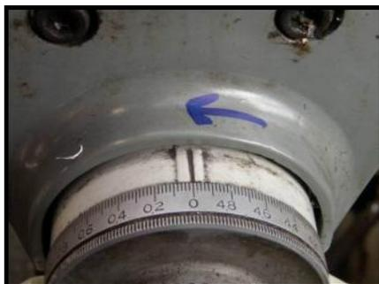
This is so as to be consistent with regard to the backlash in the nut. Not doing so will result in your work inaccurate and possibly having a faster trip to the scrap bin.
