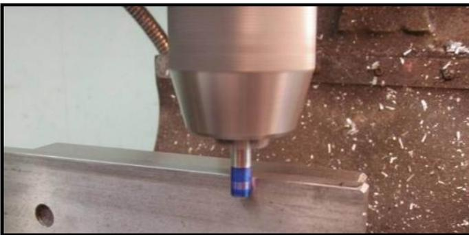
bring the dowel sideways into contact with the jaw so that ink is rubbed off the dowel and left on the jaw. The hand wheel dial is now set to zero and with the quill retracted the table is moved over by half the dowel diameter with the dials reset to zero, this is your datum 0. This process is to be repeated for the other table axis. You could also purchase a wriggler to do this job.
