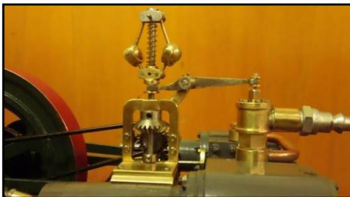
The engine could be fitted with either one or two governors. If two were fitted then the engine could have one cylinder disconnected and still run. I decided that one was more than enough. I redesigned the bed plate to make it less bulky. It now sits on a metal base 6½" by 8½" by 1½" high that sits on a wooden plinth. The engine runs very well and I am very pleased with the end result.
