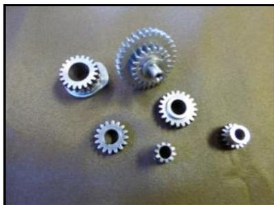
Problems arose when cam drive gears, made to plan, would not fit in the available space in the rear of the crankcase casting – bother!!
