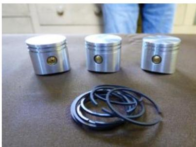
Many other parts were built, including pistons and rings, valves, special bolts, oil pump, propeller hub and spark plugs, from my last piece of ceramic tube!
