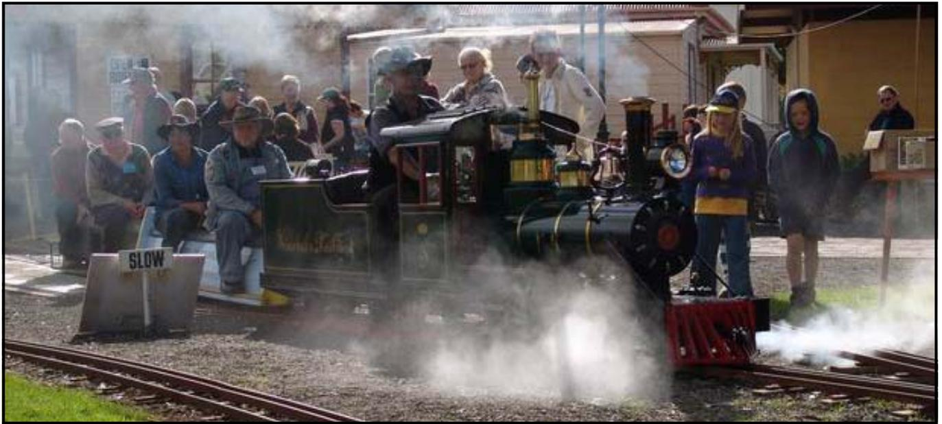
narrow gauge with the wheels inside the frames, bodywork 685mm wide.
