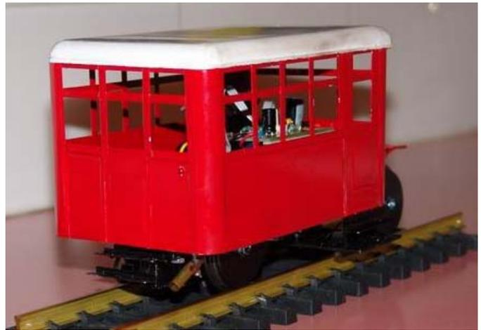
Why build a Model T railcar I hear you say? Because I could. No, not quite. I wanted to build a small G gauge loco that I could control by magnets and a microcontroller.
