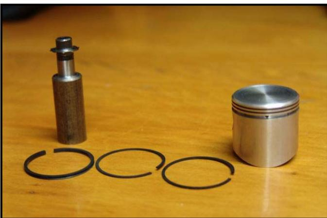
Graeme's piston, rings and the cutter used to cut the slots in the oil ring
