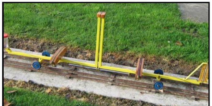
TTAFFY consists of two axles about 1.2 metres apart. One axle is attached to a steel tube and the other is attached to a bar which slides up into the tube. Each end has a level mounted near the axle and in the middle is a pair of pointers about 500mm above the frame. Each pointer is attached indirectly to the front or rear axle. These pointers greatly exaggerate the deflection between the two axles and the graduations on them are helpful in deciding the
