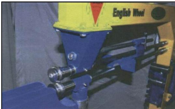
Here the wheel has been removed and the bead roller fitted.
