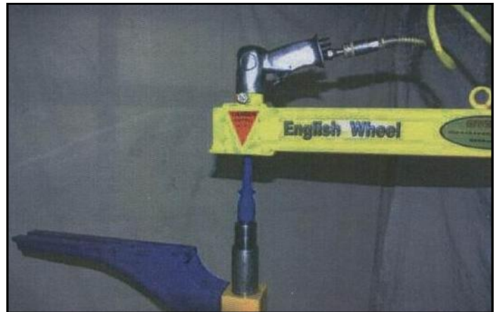
This is what the machine looks like with the blemishing hammer fitted
