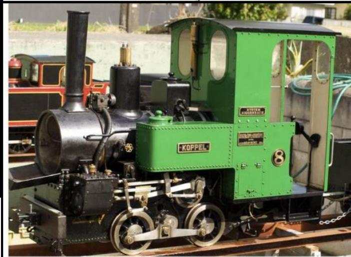
This well-presented Orenstein & Koppel geared locomotive is also fitted with Rigggenbach rack gear.
