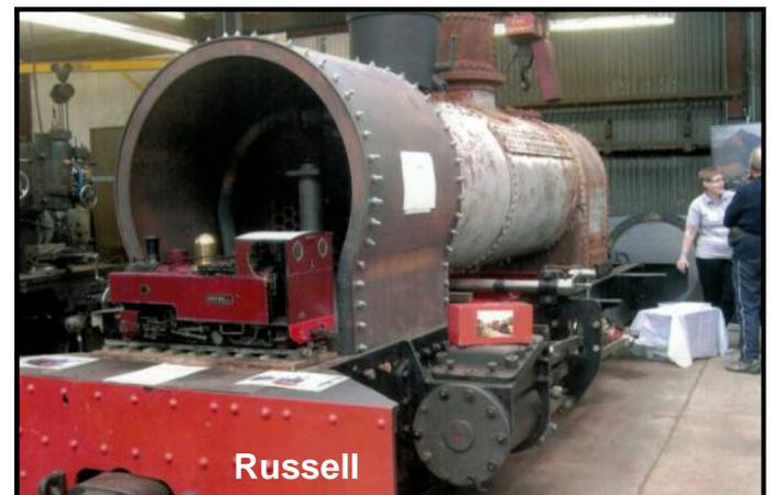
smokebox was a 3 1/2" gauge model of the Welsh engine showing what the locomotive would look like when finished.
