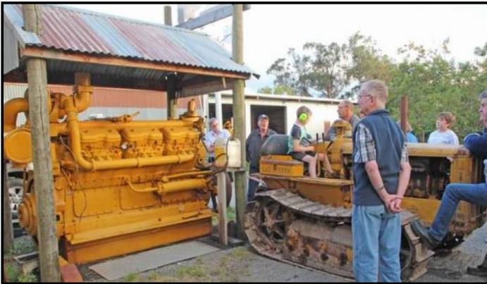
its own, the V12 was started using a flat belt driven off the power take-off on a D2 and once running the V12 had a real bellow combined with the whistle of the turbo charger. An early Chamberlain wheel tractor was started up and the three cylinder GM supercharged diesel ran very nicely. The Chamberlain is owned by a friend who doesn't have room to keep it at his place. In the collection is a John Deere MC bulldozer. These were fitted with a
