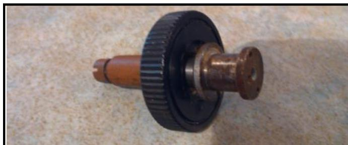
The knob on the outside seats into a recess in the body and there are three holes and a slot in the outer end. None of the holes go anywhere, the centre one is blind probably used for centering during manufacture (my guess).
