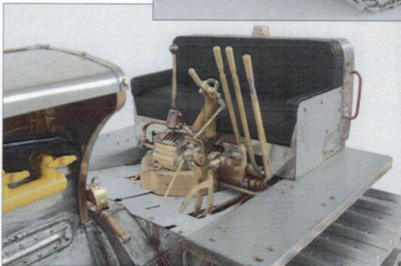
21st September 2011, All operating levers and pedals are in place and the floor plates fitted. The gear lever, master clutch and steering levers operate the tractor.
