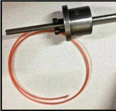
**Merv George** showed a lathe spindle back stop he had made. The stop is held in the spindle with pins that are expanded with a screw. In order to hold the pins while the backstop is being set up Merv had used pieces of plastic line from a line trimmer which provided sufficient friction to hold the pins in place while adjustments are made. It looked to be a very useful device.
