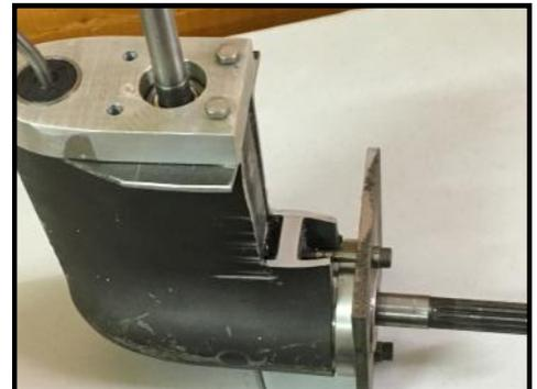
**Chris Bjerga** brought along some boiler parts for a small steam locomotive that he has been restoring. He also had a two-speed drive and gearbox from a small outboard motor which he has modified to be fitted into a 7.25” loco that will be driven by a two-cylinder Honda engine. Chris also had a partly built oscillating cylinder steam engine for a 7.25” bush locomotive.
