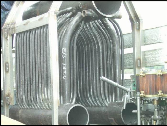
A nearly completed restoration. A White steam car of 1902. The boiler was normally fired with petrol, but the petrol – firing apparatus is not yet complete. A Propane / LPG burner has been rigged up as a temporary installation.
