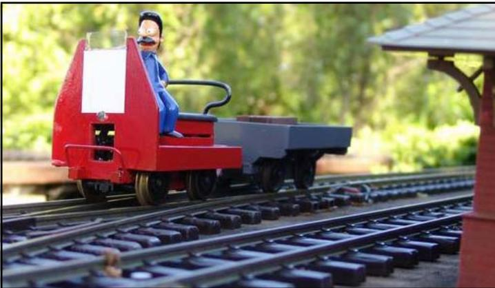
Parts were scrounged from the junk box and the drive motor from a discarded CDROM drive. The control system was hurriedly put together but I could not get it to work reliably. The software and PC board was altered and a simple remote control was used. The jigger now uses track power and infrared control giving Stop, Slow and Fast speeds.
