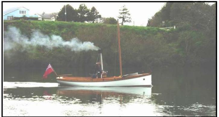
A Simpson- Strickland marine engine. Originally a two cylinder compound but the owner has fitted a third cylinder to make it a triple.
