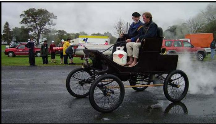
The 1902 White steam car again. This time showing some of the works. Under the seat can be seen the two high pressure cylinders. Only these very early White steam cars had twin high pressure cylinders. All their later cars had two cylinder compound engines.
