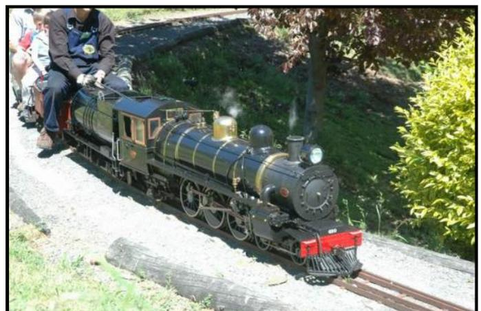
people and locomotives. On my arrival it became apparent that there was a very good assembly of 7.25 gauge NZR steam locomotives parked up in the steaming bays awaiting water and fire. There were two tender loco's, and AB and an 1874 J, both down from Auckland. Four tank loco's, W, WF, Fa and an S class single Fairlie.
