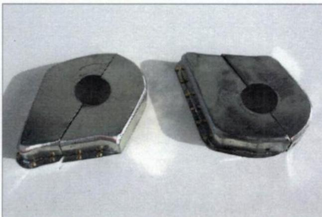
The final drive covers were made from tinfoil with dummy bolt heads soldered in as required. These were cut in half for easy removal and fitting and are held on with two screws. A puller was made to remove the half shafts allowing the complete track frame to be removed.
