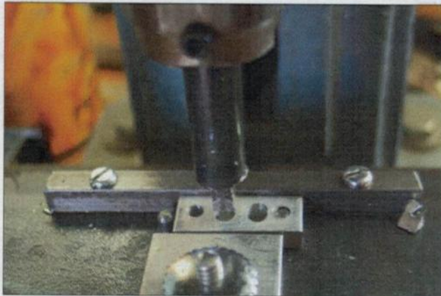
Pressing the rectangle slot in the chain link.
