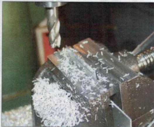
Milling the angle section on the track shoes
