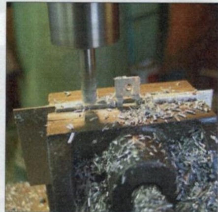
Milling the end sections on the chain link
