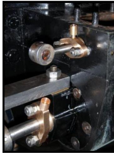
bearing journal but not so the bronze bush in the cross head. Work has also centred on the boiler with new clacks made for the injector and pump feeds to my own design raver than the prototype Kerr Stuart design with flange pipe connections which
