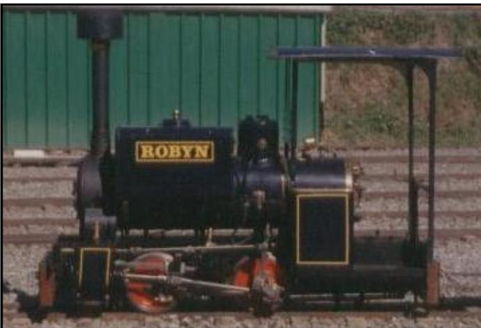
Final Version with inclined cylinders and Hackworth valve gear.
